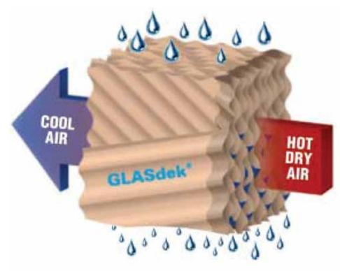
The shallow angle of Munters unequal flute design allows high velocity air to travel through the pad without significant resistance or water droplet carry over. GLASdeks' self-cleaning design resists clogging caused by dust, sand or other debris. By design, more water is directed toward the air entering face of the pad, where it flushes away dirt and debris while allowing maximum cooling performance.
