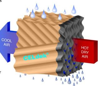
The steeper angle directs more water to the air entering side of the pad, where it is needed the most.
